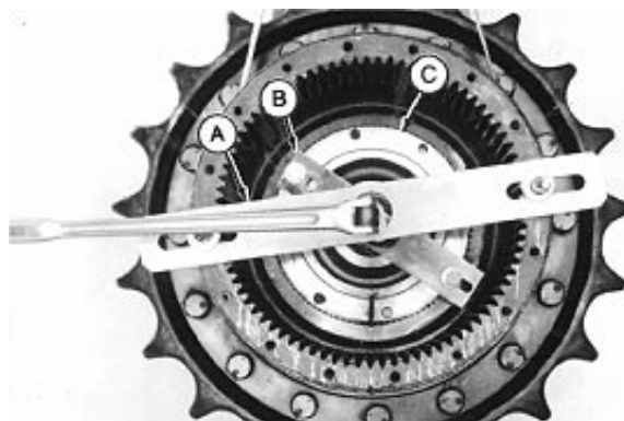
A—DFT1109 Holding Bar B—DFT1036A Propel Gearbox Nut Wrench C—Bearing Nut
