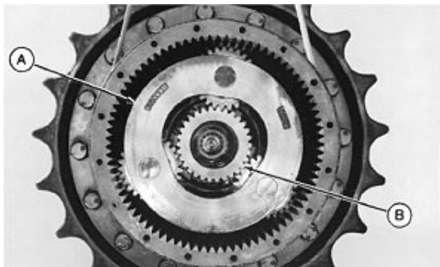
A—Third Planet Carrier B—Third Planet Sun Gear
