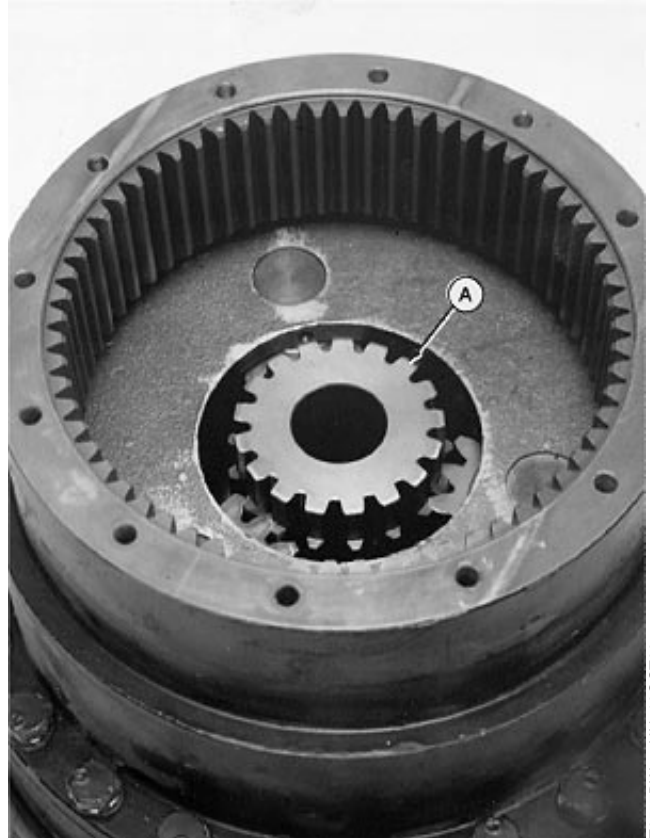
A—Third Planet Carrier and Gears
